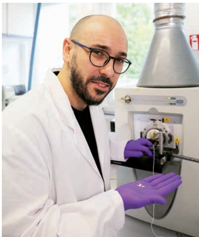
Using the mass spectrometer, Dr Marcos Bouza Areces examines animal blood samples directly on the filter paper for indications of a metabolic disorders.
