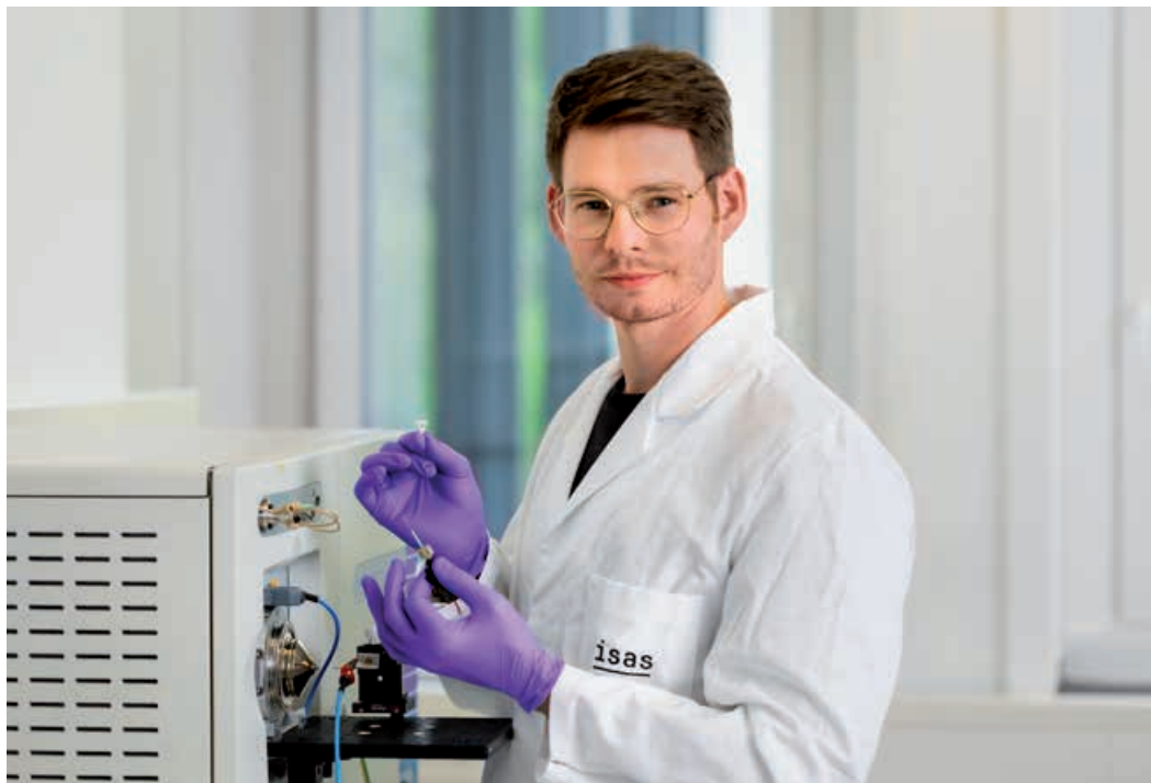
Daniel Foest is a chemist who works as a doctoral candidate in the Miniaturisation research group. In his hand, he is holding a paper with a liver sample that he is examining with the mass spectrometer using paper spray ionisation.
